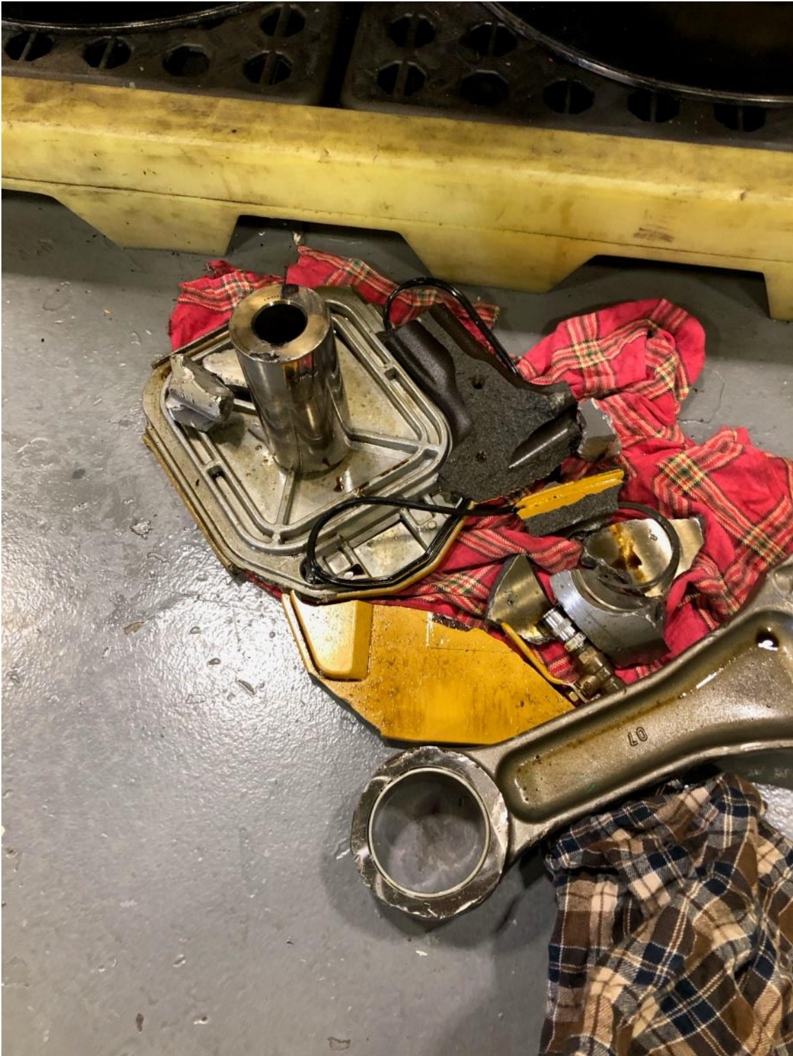
Photo A-3: Broken Pieces of Unit 2047 that were Collected, including Bent Connecting Rod, Wrist Pin, Bent Connecting Rod Bolts, Engine Block Pieces, and Piston Pieces
