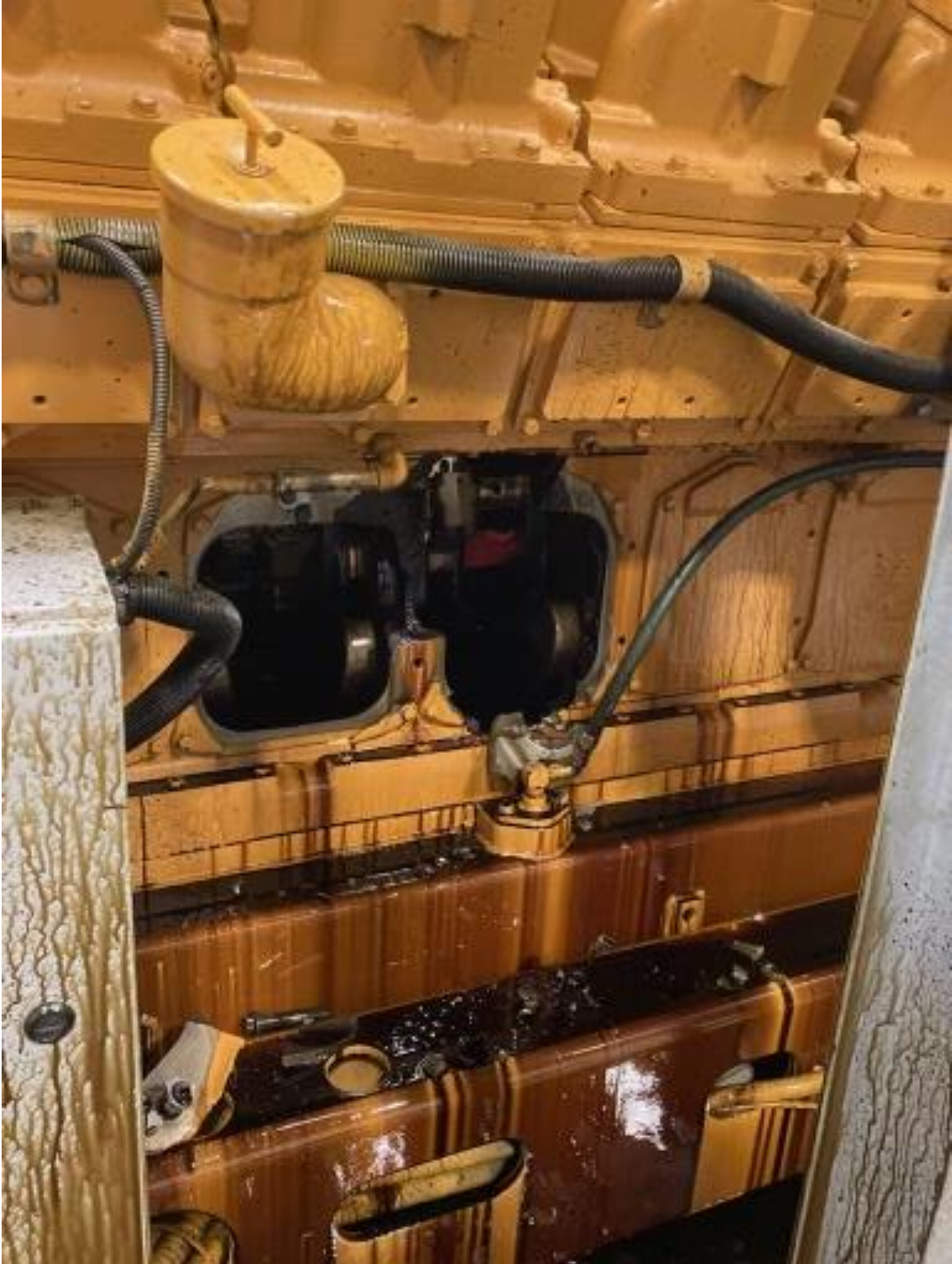
Photo A-1: Hole in Engine Block where the Connecting Rod was Ejected from the Engine
