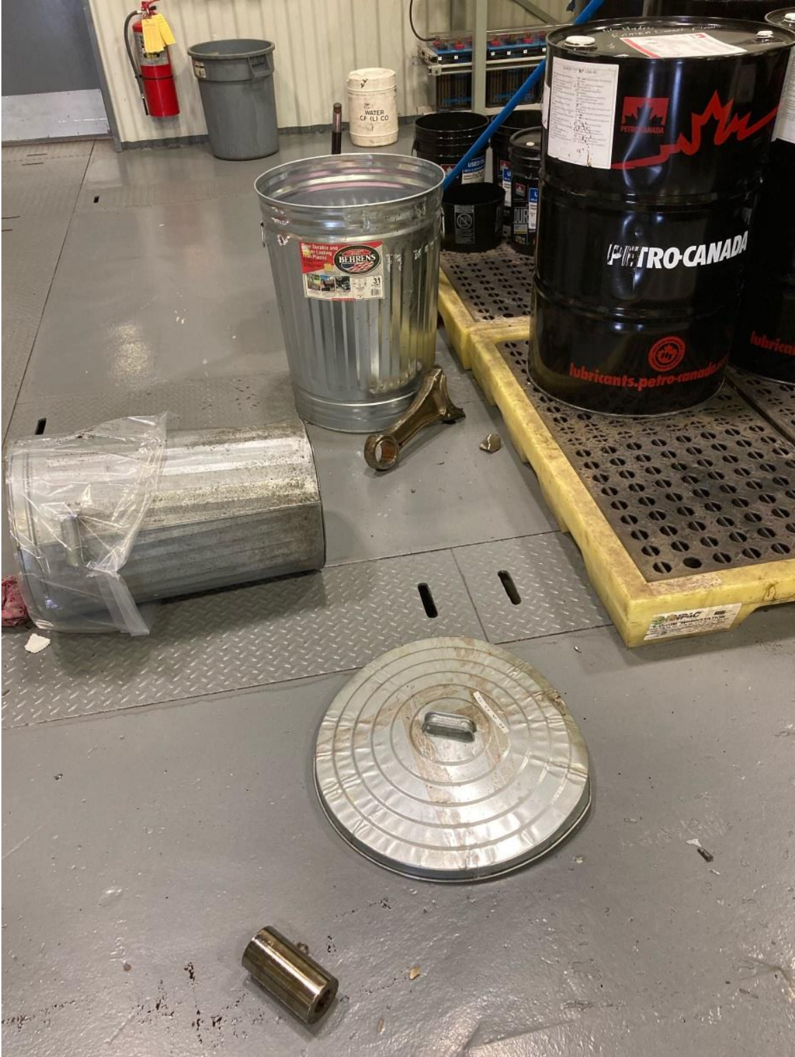
Photo A-2: Connecting Rod and Wrist Pin on the Floor after Knocking over Garbage Can from being Ejected from Engine
